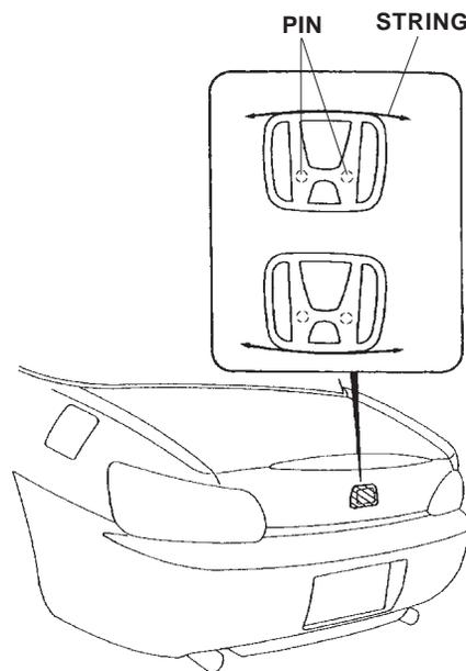
15. Remove the emblem pin inserts from the trunk lid. Using isopropyl alcohol on a shop towel, clean the area where the emblem was removed.
