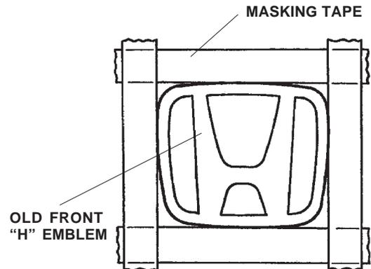
2. Using a piece of string, loosen the emblem by cutting through the adhesive backing. Move the string in the directions shown to cut the emblem free.
