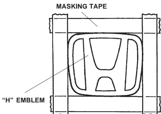
14. Using a piece of string, remove the emblem from the trunk lid. Move the string in the directions shown to cut the emblem free. Take care not to damage the body finish.
