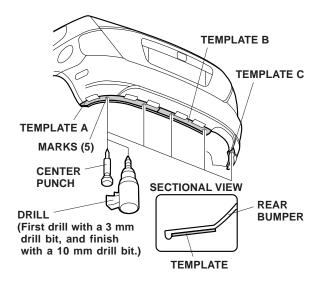
While wearing eye protection, drill a 10 mm hole through five marked locations. First drill with a 3 mm drill bit, and finish with a 10 mm drill bit. Remove all burrs from the edges of the hole with a file. 4. Using isopropyl alcohol, thoroughly clean the area where the rear under spoiler will be attached.
