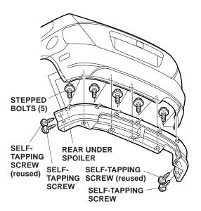
Install the four self-tapping screws to secure the ends of the rear under spoiler. Do not tighten the self-tapping screws yet. 8. Check that there is no clearance between the rear under spoiler and the rear bumper, and while holding pressure on the rear under spoiler, carefully remove the adhesive backings. When peeling off the adhesive backing, peel it off sequentially from the center of the rear under spoiler to the outside.
