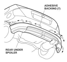
9. Attach the rear under spoiler securely by tightening the four self-tapping screws and the five stepped bolts.
