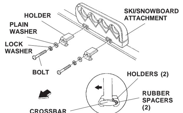
6. Insert the holder into the ski/snowboard attachment. Install one bolt with a lock washer and a plain washer into the ski/snowboard attachment and through the hole in the rubber spacer.
