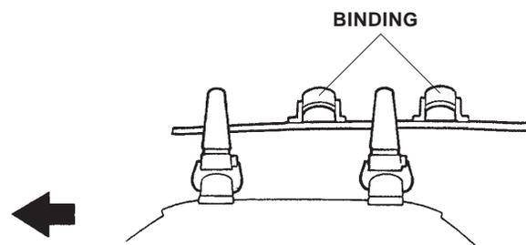
3. Close the top frame. While holding the top frame firmly against the ski/snowboard, lock the top frame by turning the key counterclockwise.
