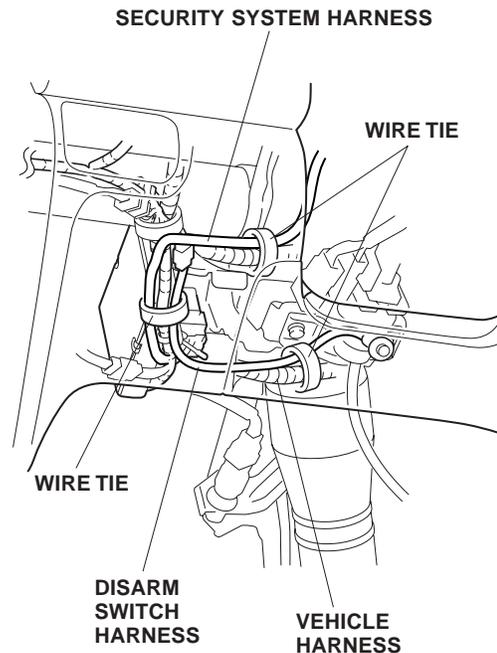
42. Check that all wire harnesses and cables are routed properly and all connectors are plugged in.
