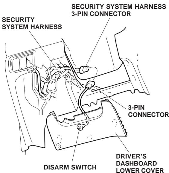
41. Secure the security system harness and the disarm switch harness to the vehicle harness with three wire ties in the areas shown.
