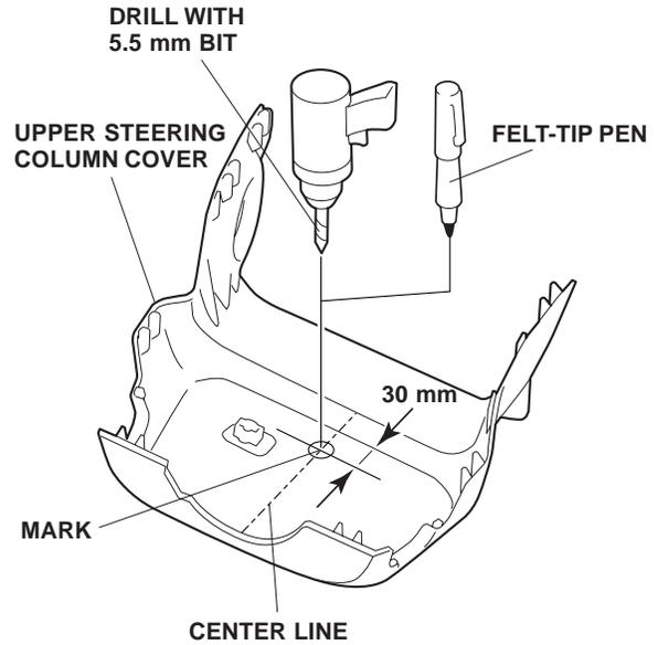
30. While wearing eye protection, lightly center-punch the mark; then drill a 5.5 mm hole through the upper steering column cover. Remove all burrs.
