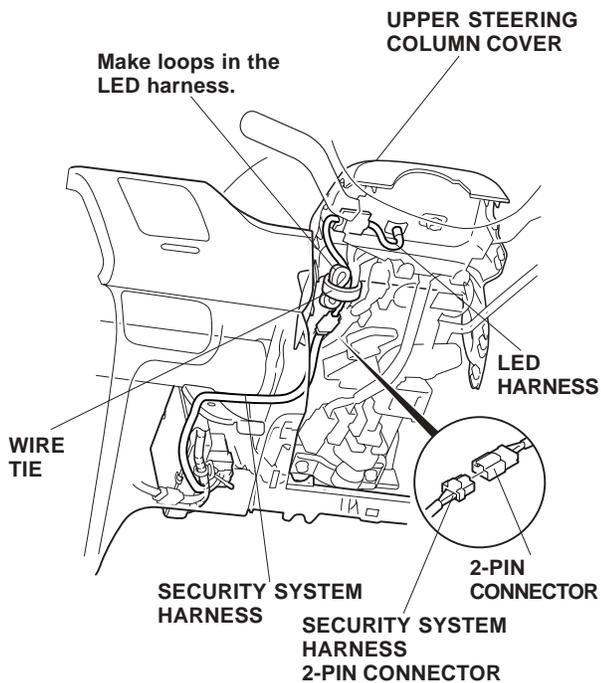
39. Make loops in the LED harness, and secure them to the vehicle harness with one wire tie as shown.
