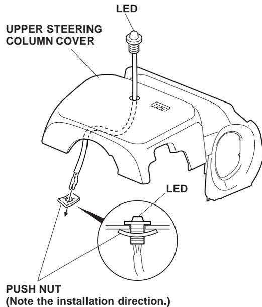
32. Using isopropyl alcohol, thoroughly clean the back of the upper steering column cover in the area shown. Secure the LED harness to the upper steering column cover with 1/2 of a cushion tape.
