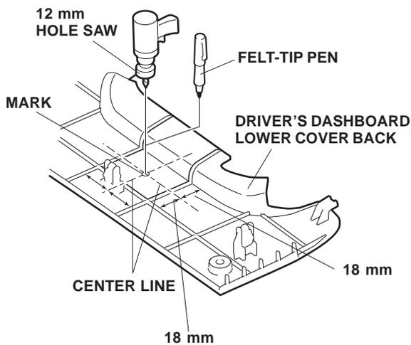
35. While wearing eye protection, lightly center-punch the mark; then drill a 12 mm hole through the center-punched mark. Remove all burrs.
