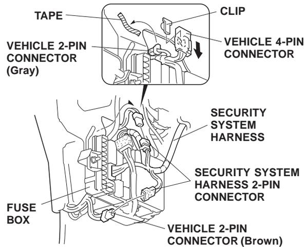
20. Below the fuse box, locate the brown 2-pin connector. Plug the security system harness 2-pin connectors into the brown connector and into the gray 2-pin connector from step 19. Reinstall the gray 4-pin connector.
