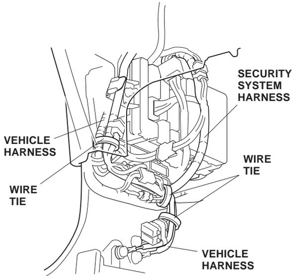
28. Further secure the security system harness to the instrument panel side frame bracket and the vehicle harness with four wire ties in the areas shown.
