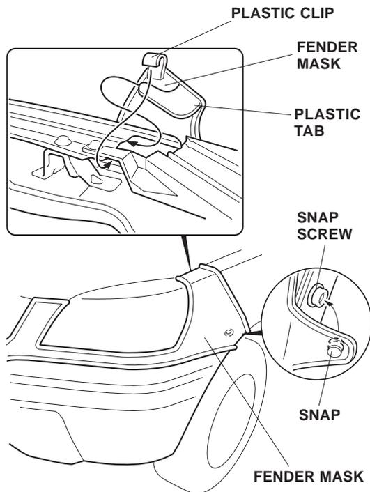
12. Pull the mask back toward the wheelwell, smooth out any wrinkles, and then snap the mask onto the snap-screw.
