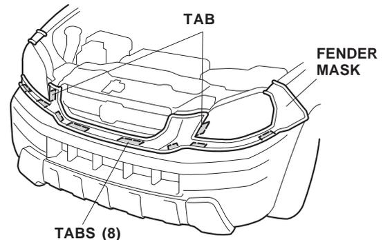
11. Slide the plastic tab of the mask's fender section into the opening at the front corner of the fender, then attach the plastic clip to the top inside edge of the fender. Fit the mask across the bumper.
