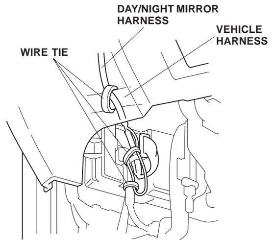
32. Check that all wire harnesses are routed properly and all connectors are plugged in.
