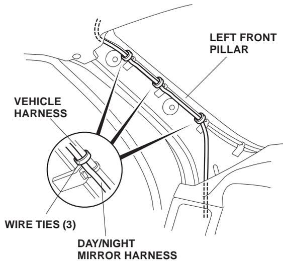
30. Using isopropyl alcohol on a shop towel, clean the area where the cushion tape will attach. Secure the day/night mirror harness to the left front pillar with one cushion tape in the area shown.
