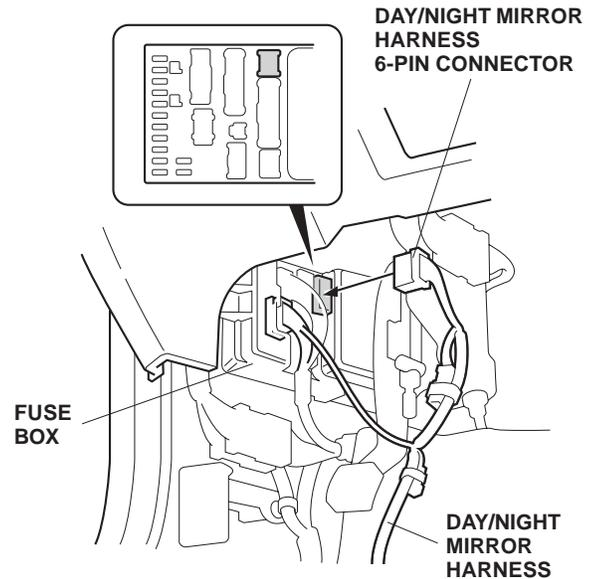
NOTE: If you are also installing the fog lights, remove the dummy connector from the 6-pin connector taped to the day/night mirror harness. Connect the 6-pin connector of the fog light to the 6-pin connector you just unplugged as shown.
