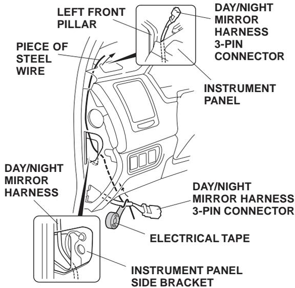
24. Remove the electrical tape and the steel wire from the day/night mirror harness.
