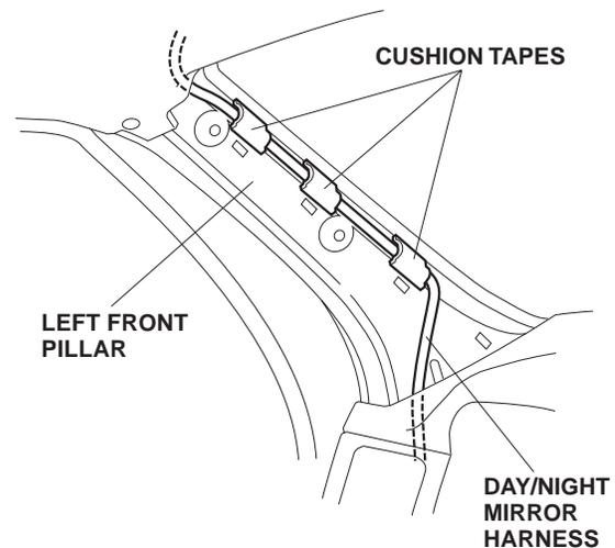
29. **With RES;** after the vehicle harness is routed along the left front pillar, secure the day/night mirror harness to the vehicle harness with three wire ties in the areas shown.
