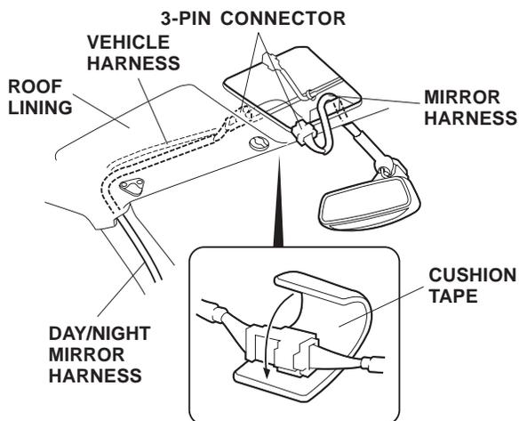
26. Connect the day/night mirror harness 3-pin connector to the 3-pin connector of the mirror harness. Wrap one cushion tape around the connectors.
