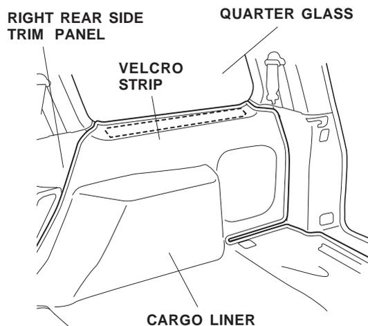
16. Remove the adhesive backing from the Velcro strip, fold the cargo liner over, and attach the strip to the right rear side trim panel. Press the Velcro strip firmly against the trim panel with the palm of your hand.
