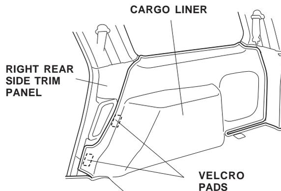
14. Remove the adhesive backing from each Velcro pad. Press the Velcro pads firmly against the right rear side trim panel with the palm of your hand.
