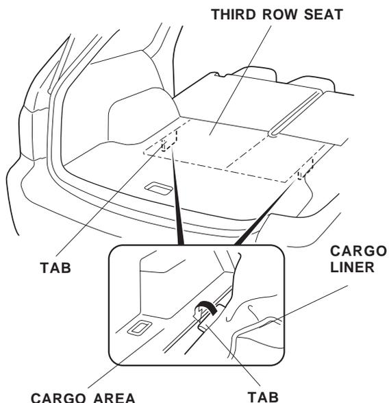
11. Open the cargo area floor lid, and fit the pocket of the cargo liner around the floor lid. Using one alcohol wipe, clean the area where the Velcro pads will attach.
