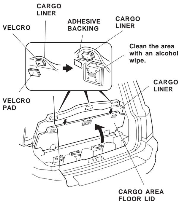
12. Remove the adhesive backing from each Velcro pad, and attach the Velcro pads to the storage compartment cover. Press the Velcro pads firmly against the cover with palm of your hand.
