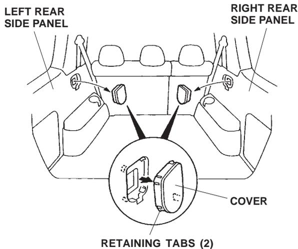
6. Install the cargo cover into the recess in the left rear side panel in the direction shown, then compress the cargo cover, and install it in the right rear side panel.
