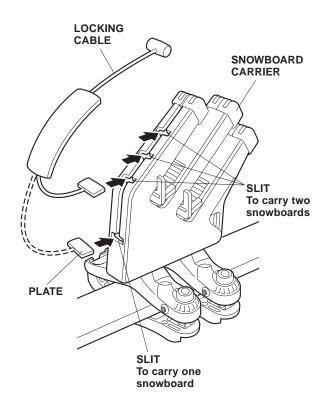
15. After loading the snowboard(s) on the carrier, adjust it (them) with the help of the board supports so that the top edges are level and the boards are as far down in the carrier as possible. To secure the snowboard(s) use the key to open the covers, and insert the locking cable stoppers into the holes of the carrier covers.
