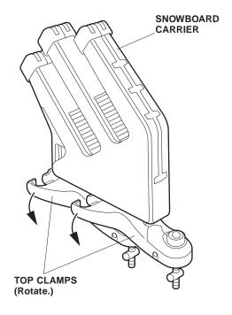
2. Install two board supports on the snowboard carrier.
