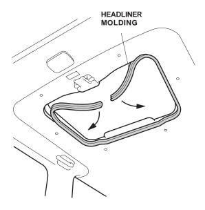
10. Gently pull down the headliner and install one snap screw, two washers, and one flange nut through each of the six holes you made in the headliner.
