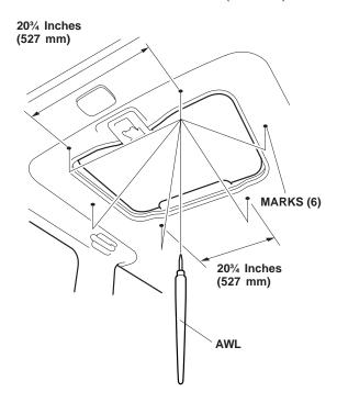
6. Using an awl, make a hole through the headliner at each of the six marks on the headliner.
