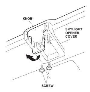
8. Disengage the tab and remove the skylight opener cover.
