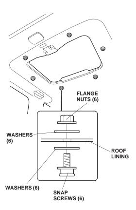
11. Reinstall the molding placing it over the roof panel and roof liner.
