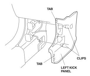
9. Remove the right kick panel (pull to release the two clips).
