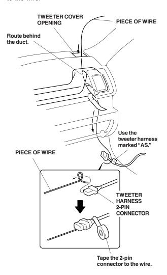
21. Pull the right tweeter 2-pin connector up from the floor to the tweeter cover opening.
