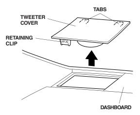
8. Remove the tweeter cover from the right side of the vehicle using the above procedure.
