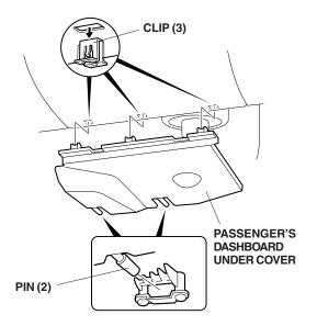
4. Open the glove box. Release the right and left stops.
