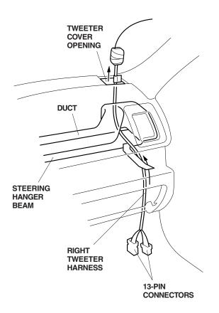
22. Remove the wire from the 2-pin connector. To prevent the tweeter harness from falling, tape it to the dashboard.
