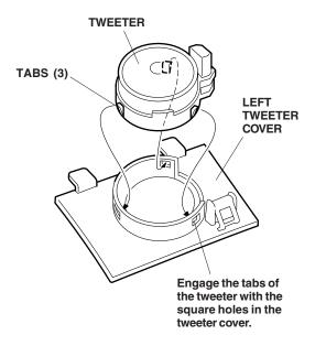
17. Plug the left tweeter harness 2-pin connector into the tweeter 2-pin connector, then reinstall the tweeter cover.
