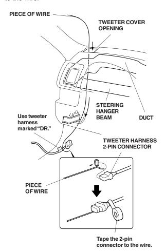
13. Pull the left tweeter harness 2-pin connector up from the floor to the tweeter cover opening.
