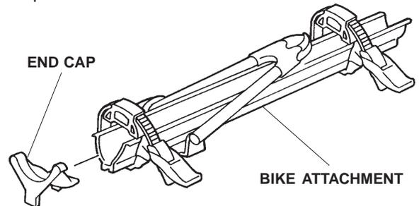
3. Turn and loosen the mounting levers on the bike attachment.
