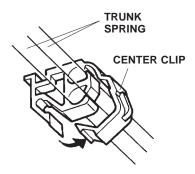
14. With an assistant holding the trunk lid open, remove the old trunk springs from the trunk hinge arms using the special tool. Wear gloves to protect your hands, and pull the special tool slowly and carefully toward you.
