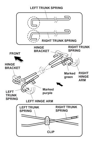
16. Reinstall the center clip on the trunk springs.
