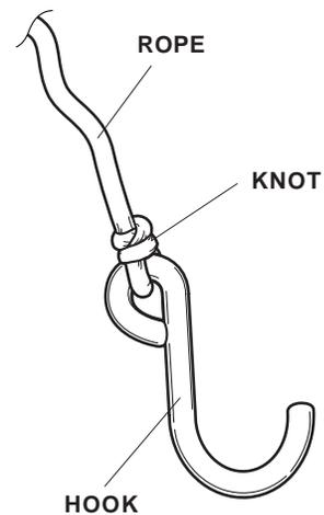
10. Route the other end of the rope through the bottom of a ratchet hook in the direction shown, and turn the spool until the rope end comes out of the ratchet.
