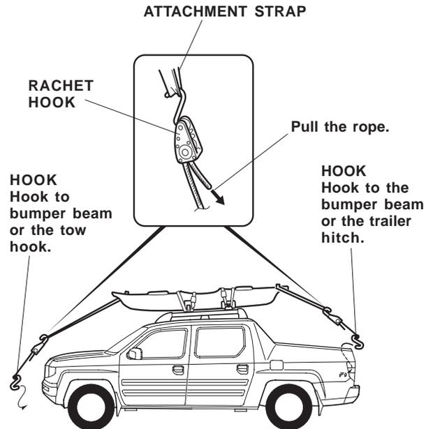
13. To loosen the rope, push up on the ratchet strap lever, then pull on the rope.
