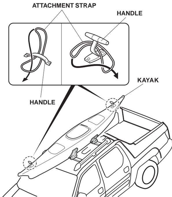
12. Attach one ratchet hook to the front attachment strap and one ratchet hook to the rear attachment strap. Attach the front hook to the front bumper beam or to the tow hook. Attach the rear hook to the rear tie-down anchors in the bed. Secure the kayak to the vehicle by pulling the rope through the ratchet hooks.
