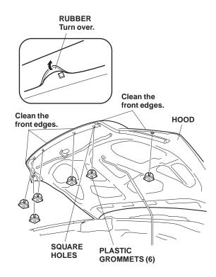
Clean the front edge of the hood with the other alcohol pad from the kit. 6. Slide the front brackets A and B and the side brackets over the lip of the hood. Align the hole in each bracket with the hole in the plastic grommet.
