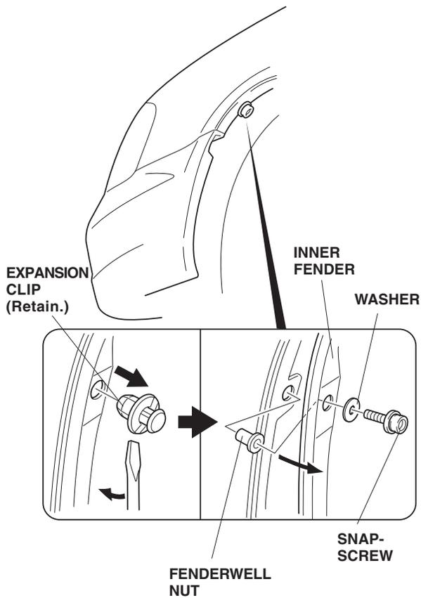
5. Pull the inner fender away, and press one fenderwell nut (supplied) into the hole in the fender flange.
