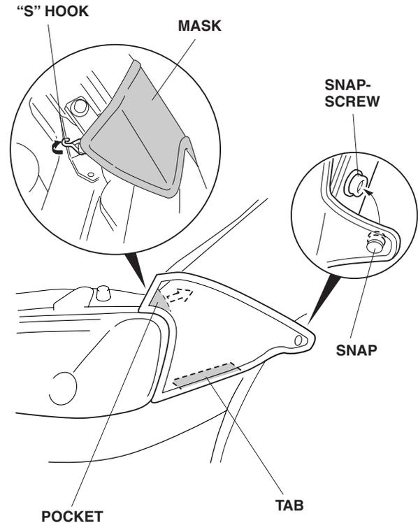
9. Pull the mask back toward the wheelwell, smooth out any wrinkles, and then snap the mask onto the snap-screw.
