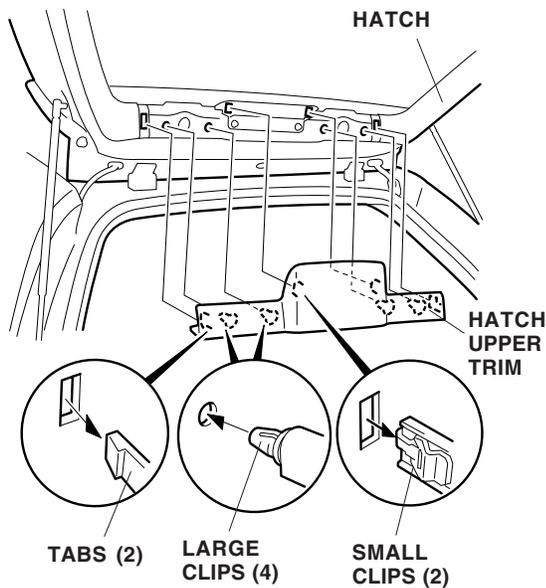
2. Remove the side trims by pulling the right and left side hatch trims out toward you (two large clips and one tab).
