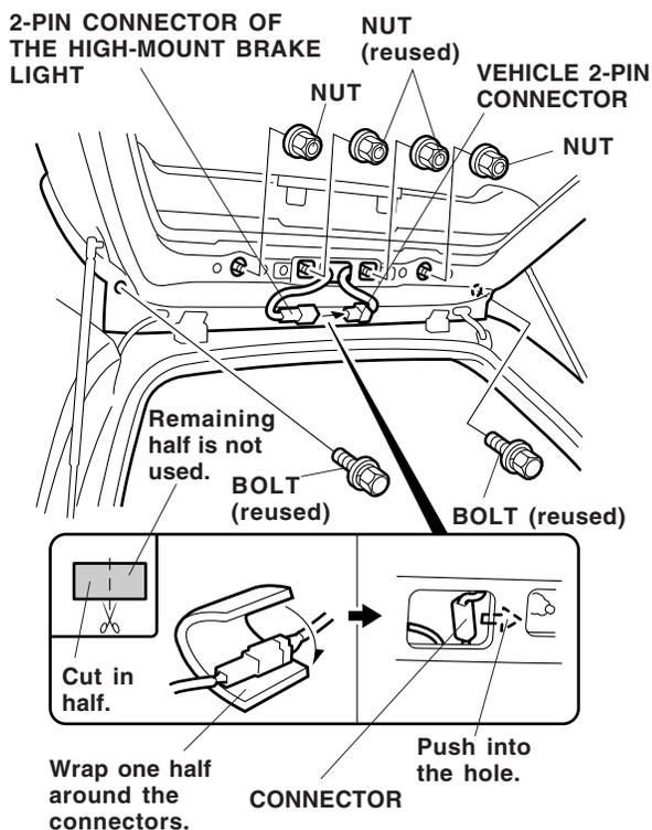
26. Connect the high-mount brake light 2-pin connector into the 2-pin connector of the vehicle harness. Cut the EPT sealer in half, wrap one half around the connectors, and push them into the center hole of the hatch. (The remaining half of the EPT sealer is not used.)
