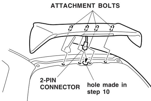
25. While holding the hatch spoiler in place with one hand, open the hatch with your other hand; secure the spoiler with the two bolts and four nuts. Torque the nuts to 8.8 N·m (6.5 lb-ft).
