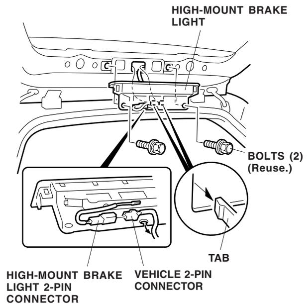
4. Disconnect the 2-pin connector on the rear of the high-mount brake light from the vehicle 2-pin connector, and remove the high-mount brake light from the hatch.
