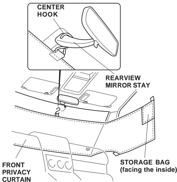
3. Spread the privacy curtain over the right side of the front windshield and passenger's window. Slide the front tab between the the dashboard and the A pillar and slide the other tab between the rear door striker cover and the headliner.
