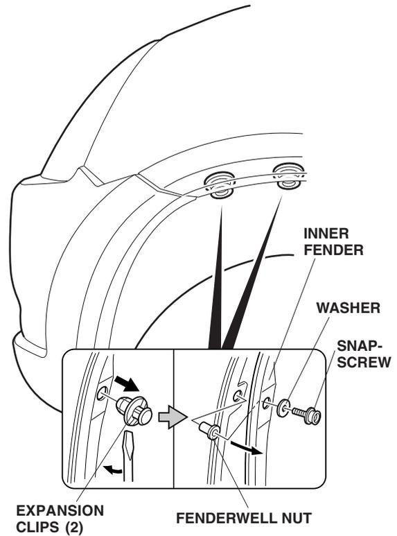
5. Pull the inner fender away, and press two fenderwell nuts (supplied) into the holes in the fender flange.
