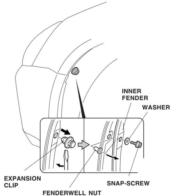
7. Pull out on the inner fender, and press one fenderwell nut into the hole in the fender flange.
