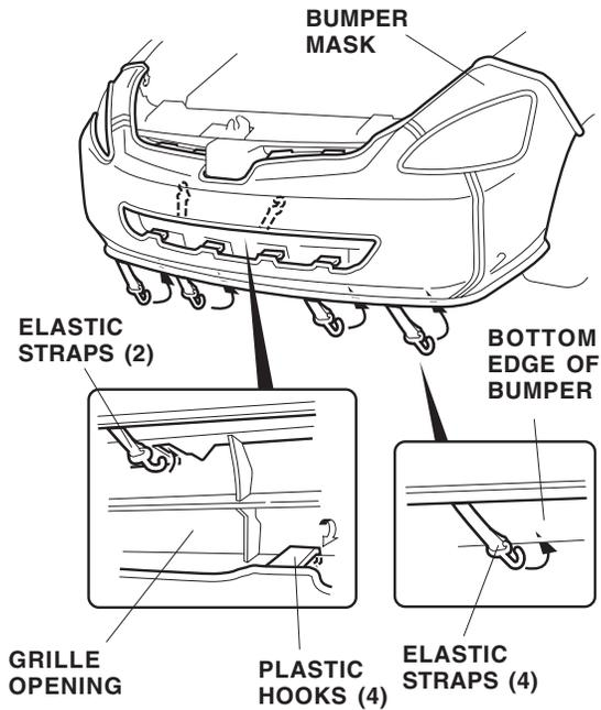
16. Attach the four remaining elastic straps to the bottom edge of the bumper.
