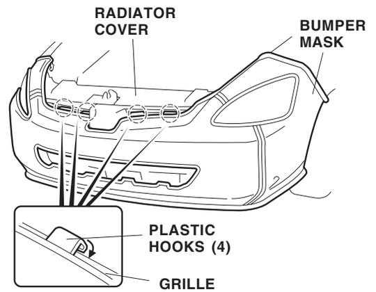
15. Attach the two elastic straps to the inside top edge of the grille opening, and attach the four plastic hooks to the bottom inside edge of the grille opening.
