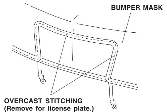
2. If the car you are working on is equipped with fog lights, cut out the piece of the bumper section that covers the fog lights:
