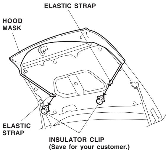
4. Fit the corners of the hood section around the hood, and adjust the mask so it fits smoothly over the edges. Attach the two elastic straps to the holes in the hood.
