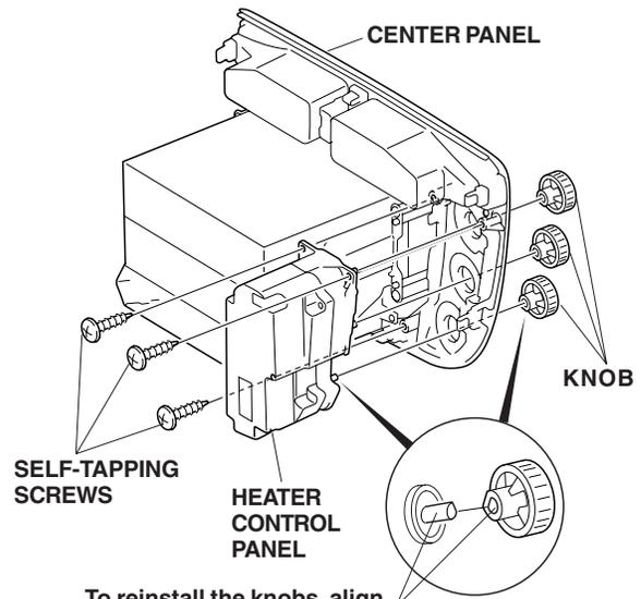
To reinstall the knobs, align the flat surface on the rod with the flat surface on the hole of each knob.
