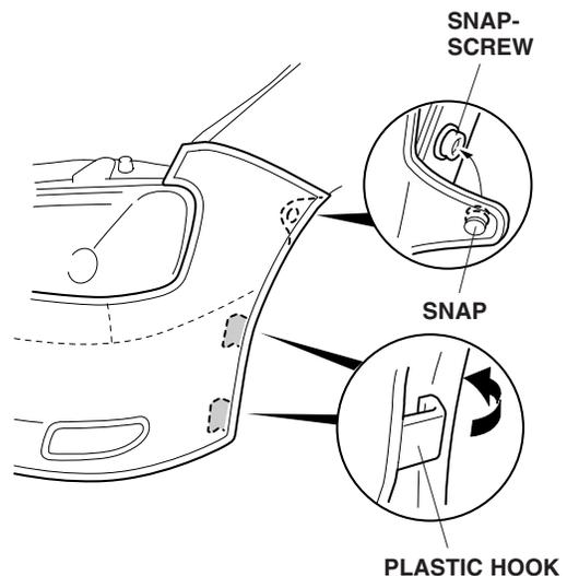
10. On both sides of the vehicle, attach the two plastic clips to the fenderwell.
