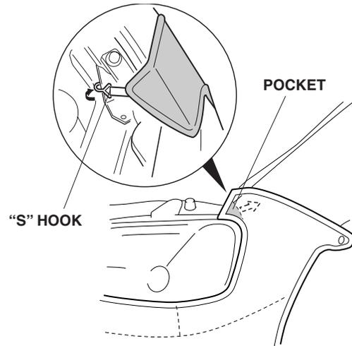
9. Pull the mask back toward the wheelwell, smooth out any wrinkles, and then snap the mask onto the snap-screw. Repeat on the other side.
