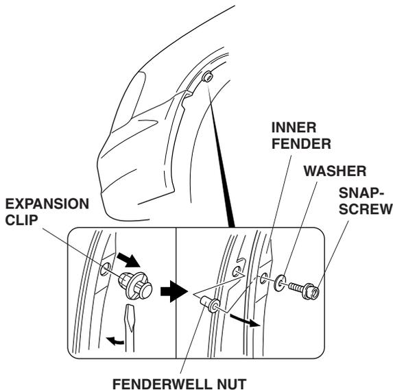
5. Pull the inner fender away, and press one fenderwell nut (supplied) into the hole in the fender flange.
