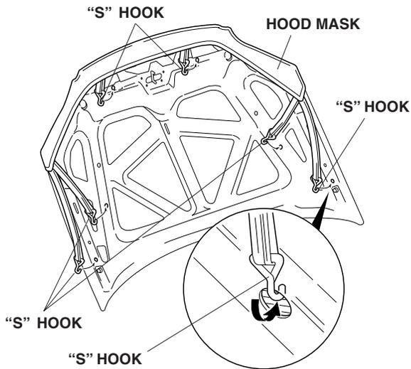
2. Secure the mask by hooking the six "S" hooks to the holes in the back of the hood.
